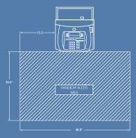
The dimensions shown comply with US Federal ADA guidelines. For installation within the US, be sure to check state and local guidelines for complete compliance. For non -USA installations, check regulations for the country in which the machine will be installed. For additional information on any of the ATMs in Triton's line-up, please visit our website at www.tritonatm.com.
